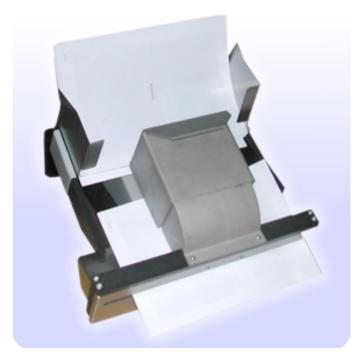
A high performance variable thickness feeder for filled and sealed envelopes and booklets, offering patented singulation technology and capable of processing up to 16,000 items per hour
